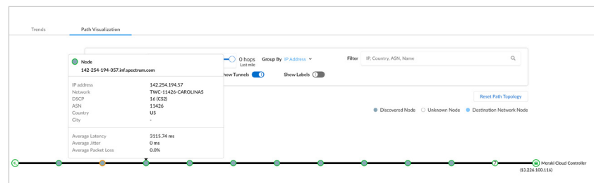
Figure 11: Hop-by-hop path visualization for remote networks on a direct access path
