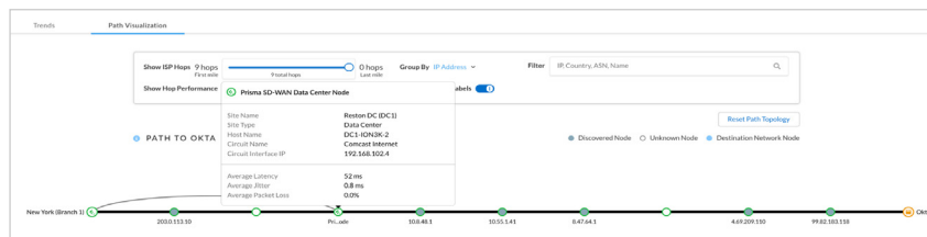
Figure 12: Hop-by-hop path visualization for remote networks on a Prisma SD-WAN path
